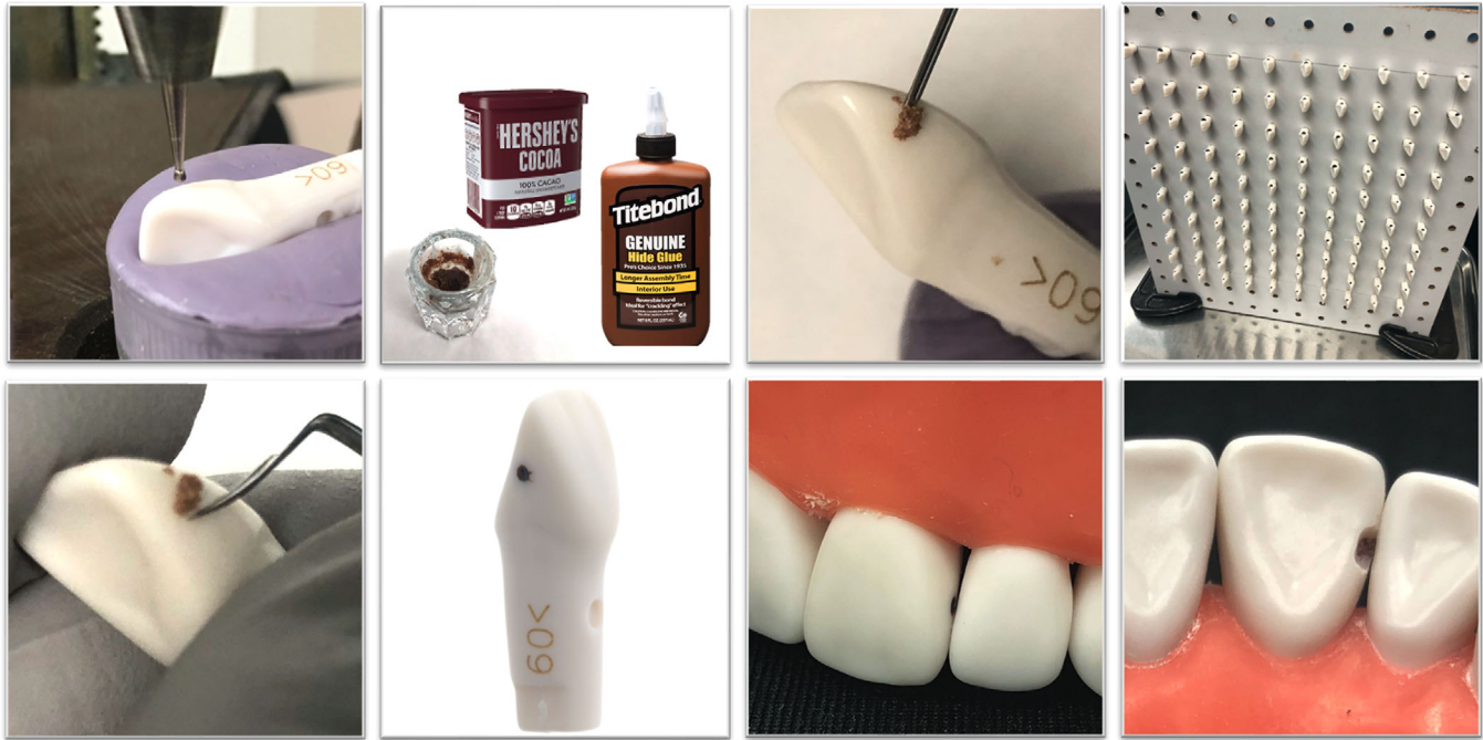
FIGURE 1 ACT fabrication sequence and usage in preclinical operative training. (A) A Craftsman drill platform was equipped with a straight handpiece bur to standardize the location with a depth of 1.25 mm and diameter of 1 mm on the distal surface of #9, ModuPro typodont tooth. (B) Artificial caries was made with Titebond Hide glue mixed with chocolate powder in 10:1 weight ratio, respectively. (C) A small injection syringe was used to insert the mixture into the cavities. (D) Teeth were mounted on a spacer board, made to hold at least 100 teeth, for the glue mixture to set. (E) A Hollenbeck carver was used to remove excess flash that was present after drying. (F) Completed ACT of #9. (G) ACT mounted on typodont showing the artificial caries when viewed from the facial. (H) Initiation of the Class III cavity preparation with artificial caries remaining on the facial wall.
