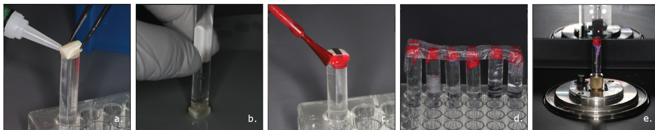
Figure 2. Step-by-step protocol for micro-CT erosion assessment. (a) Sample mounting; (b) Sample polishing; (c) Varnish painting; (d) Whitening treatment; (e) Micro-CT scanning.
